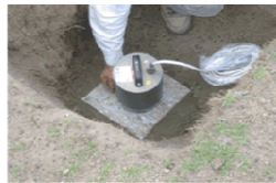
2- Deployment of seismometer on top of a concrete plate
