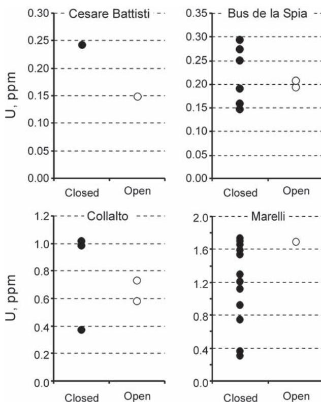
Fig. 5 - Comparison of U contents in samples from the same caves, data from which show both closed- and open-system behavior (data from Tab. 2).
