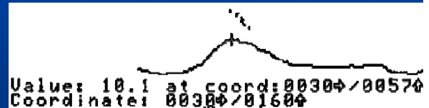
When passing over a conductive structure WADI display shows a peak.
