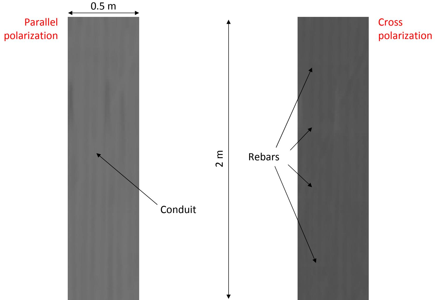
The scan is perpendicular to the corrugations. The transversal conduit is only visible by RASCAN; a 60Hz live power line detector showed no response.
