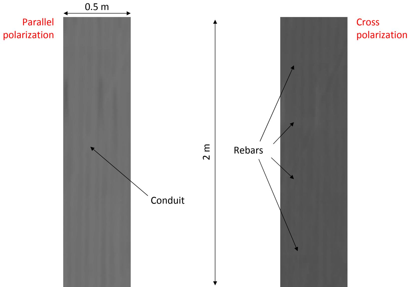
The scan is perpendicular to the corrugations. The transversal conduit is only visible by RASCAN; a 60Hz live power line detector showed no response.
