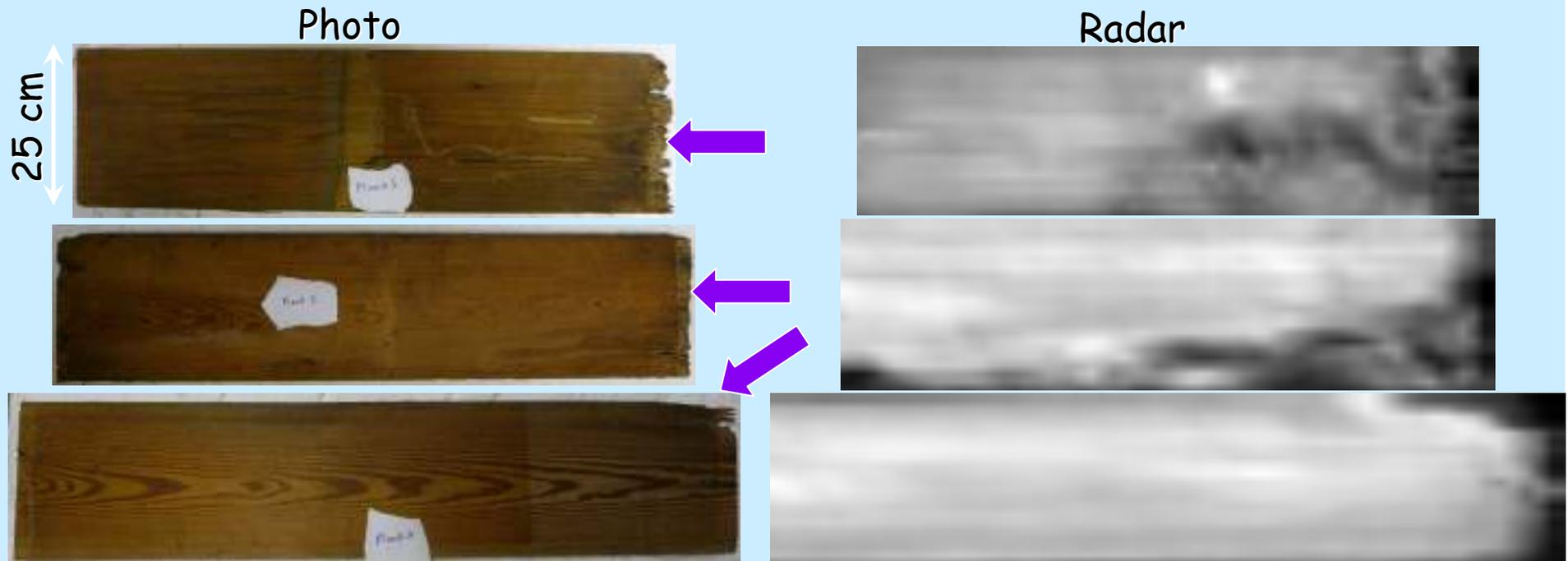
Tunnels visible on edge of boards only, but radar reveals internal variations also.
