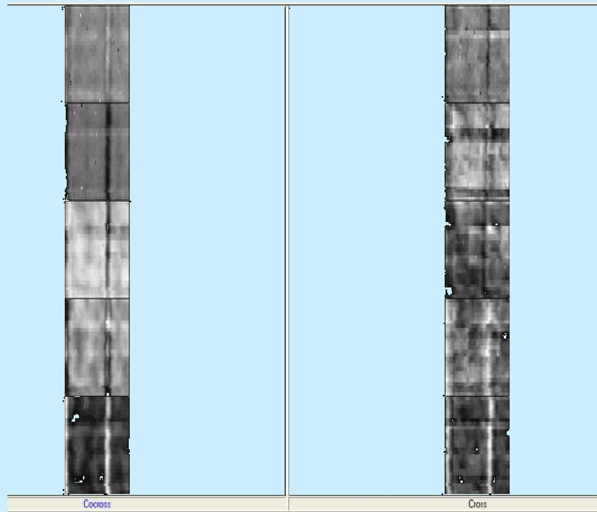
The cocross images show clearly the vertical metal bar on the left and the horizontal joint layers between concrete blocks on the right.
