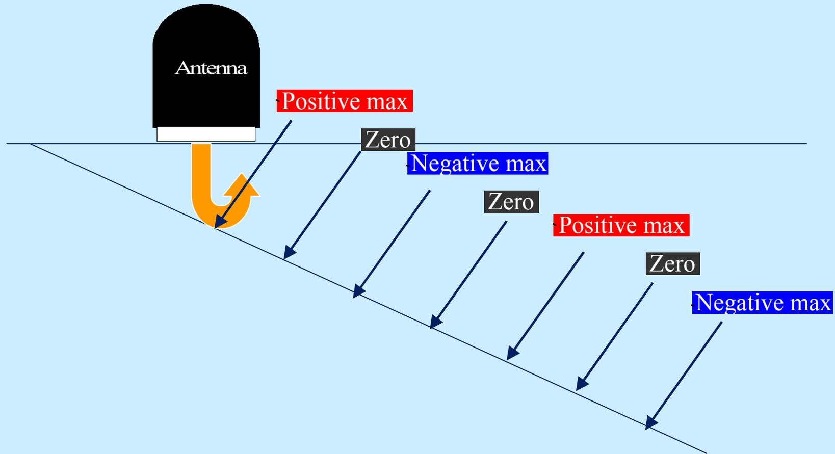
To avoid blind spots holographic radar works with  $N$  discrete and programmable frequencies
