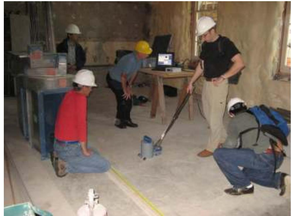
Scan on floor surface with RASCAN 2 GHz
