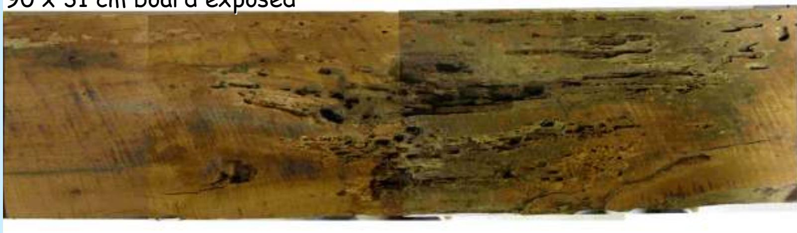
Radar image recorded through 1 cm plasterboard
