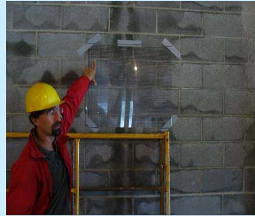
Scanning the wall by using a ruled plastic mat. Wet spots are present
