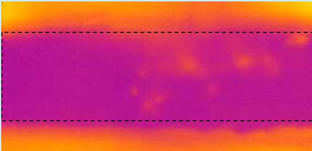
FLIR i60 image recorded through 1 cm plasterboard, with space heater behind board. Appearance of damage is transient only.
