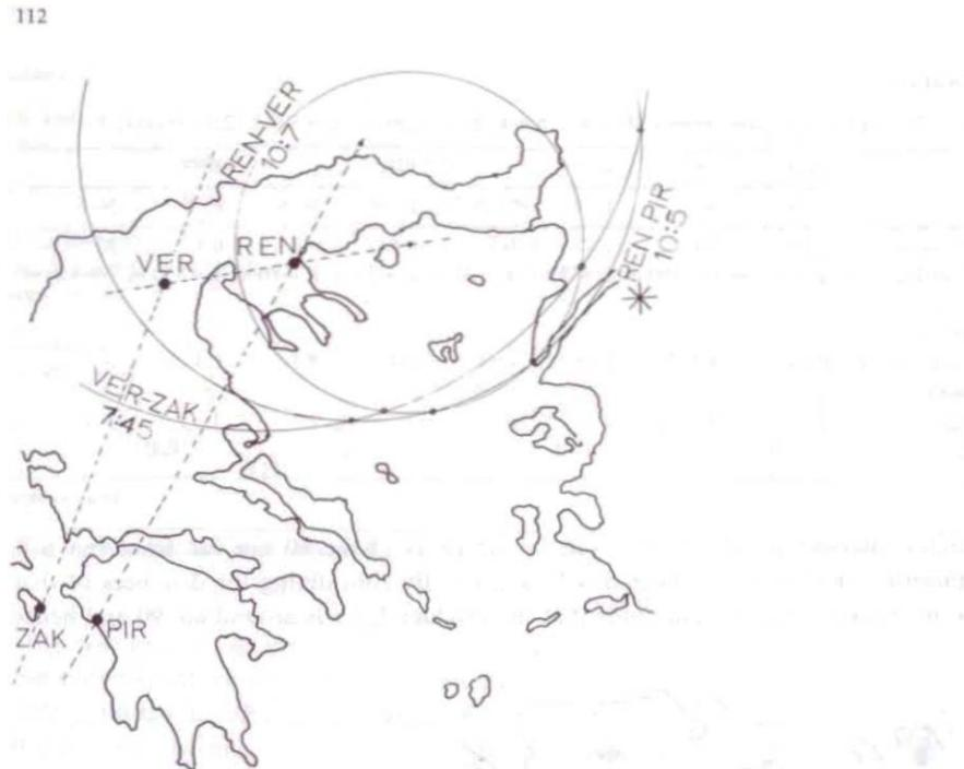
Fig. 13. Graphical determination of the epicenter of the  $M = 6.5$  event that occurred at 12:01, July 5 in the Dardanelles. The SES was recorded at REN, VER, ZAK and PIR. The Apollonian circles correspond to the pairs of stations denoted in the figure. The star shows the true epicenter and solid circles the predicted epicenter from the intersection of the circles.
