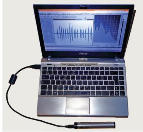
Fig. 3 - The ultrasound-recording apparatus including the Ultramic 250 microphone and the Asus Netbook portable computer.
